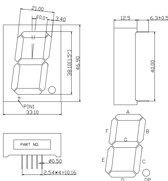
NOTES: All dimensions are in millimeters (inches) tolerance are  $\pm 0.25\text{mm}(0.010)$  unless otherwise noted.
